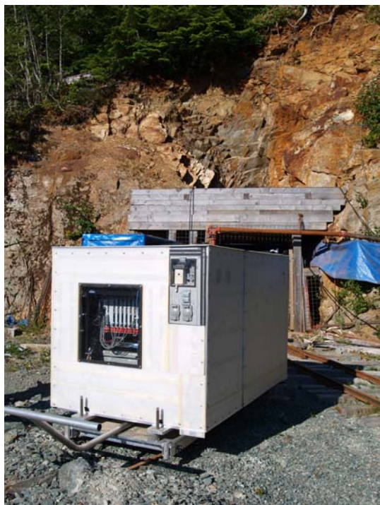
Figure 4. Muon sensor enclosure on a rail cart prior to entry into the mine tunnel.
